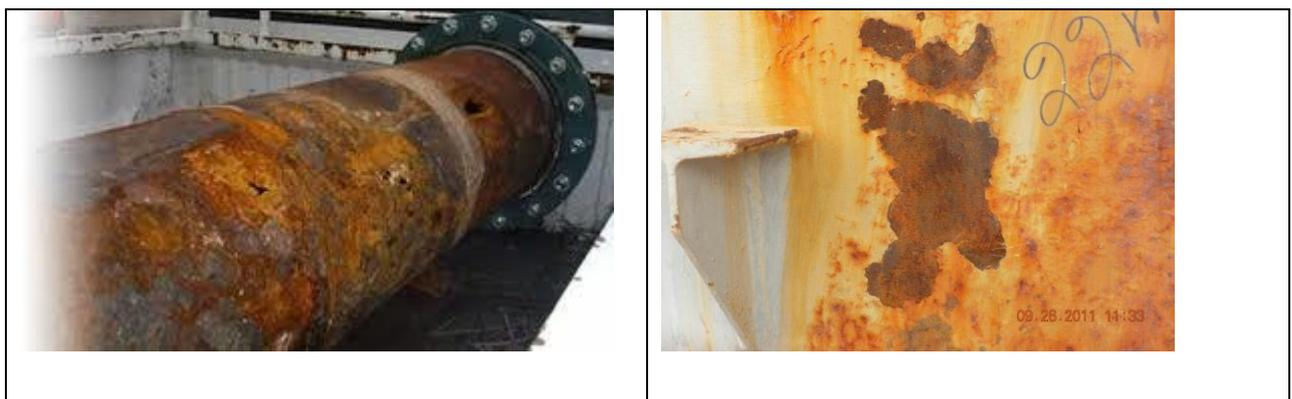
Corrosion can be a problem in air, but it is a far more significant issue in seawater. Here the process is initiated by the presence of oxygen and greatly exacerbated by the prevalence of chlorides, which makes the seawater an excellent conductor.
